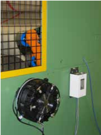
The ionisation power unit mounted on the side of the machine.
