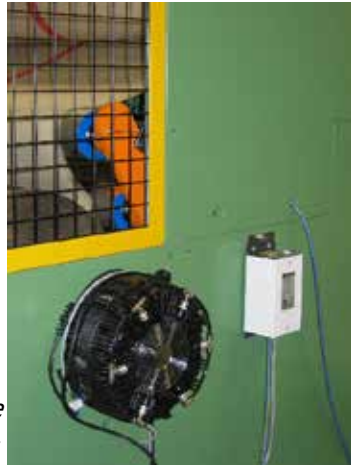
The anti-static bar, showing an electrode and cabling.
